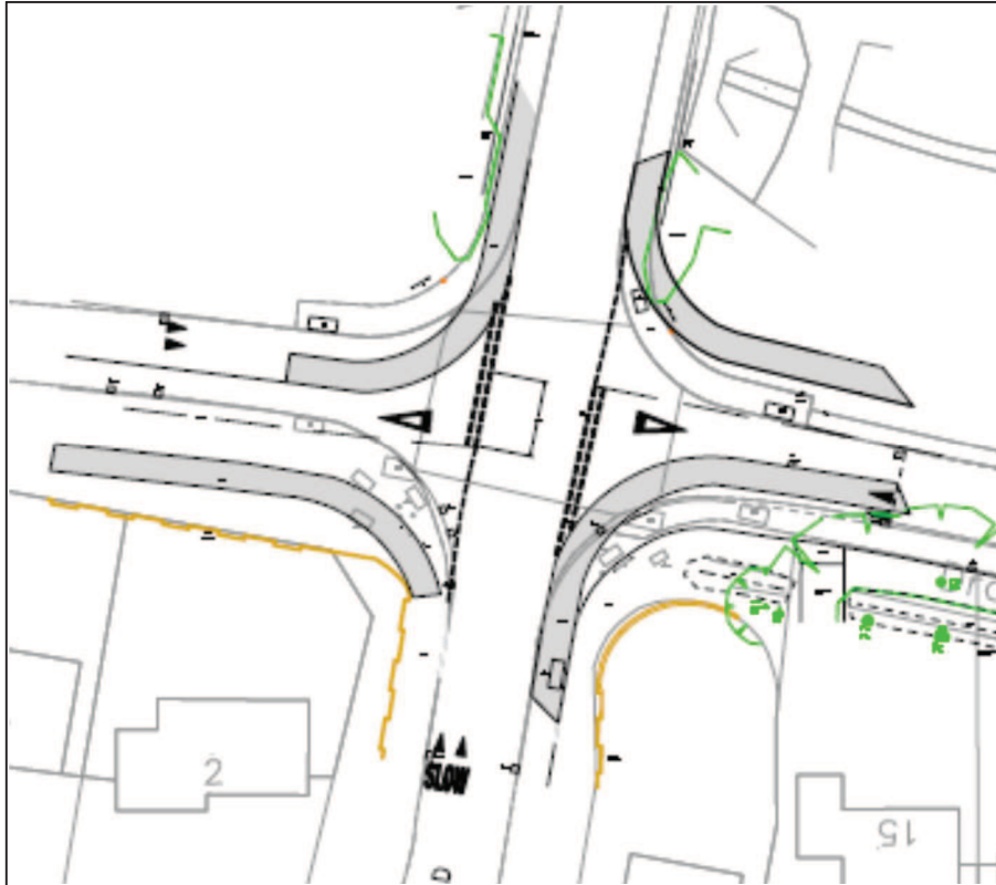
Figure 10.3 – Option 3: Change priorities and introduce a stagger on Langshott (to get full benefit in terms of blocking visibility stagger would be the other way)
